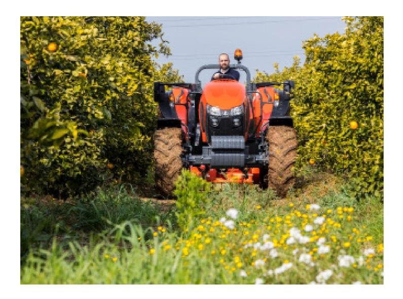
A tractor often requires no cabin. That's where the ROPS version of the M5002 is the ideal choice. This tractor, with its open platform and rollbar, enables you to get on and off quickly on both sides thanks to its flat floor and the absence of doors. Kubota provides this tractor with a electrohydraulic shuttle reverser and 18 forward and reverse gears, which can be shifted very smoothly.
